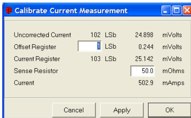
To calibrate DS2438 current measurements for offset error, follow these steps:
