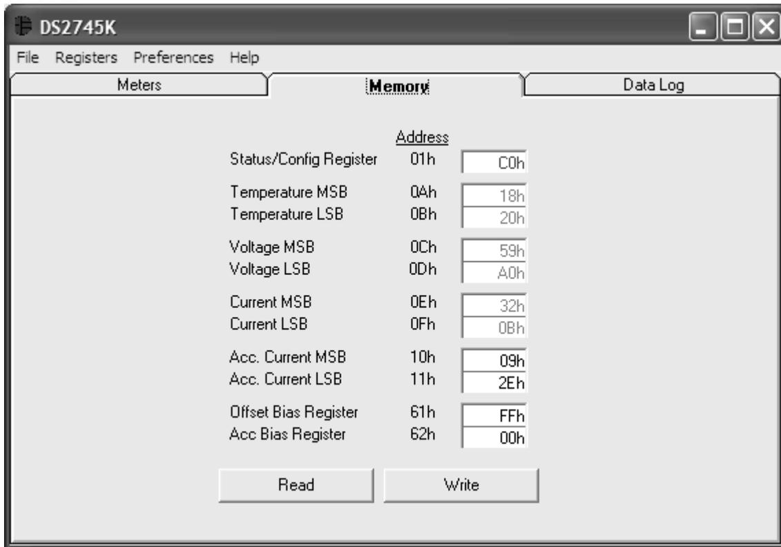
The Memory Tab gives the user access to all 11 bytes inside the DS2745. The WRITE button will write the Status Register, the Accumulated Current Register, the Offset Bias Register and the Accumulation Bias Register. The Read button reads all of the bytes shown.
