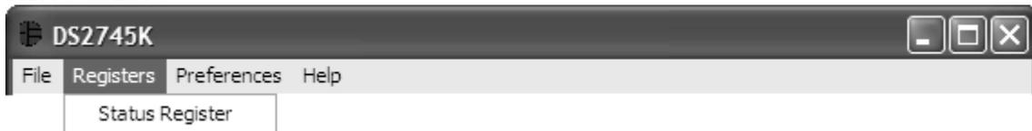
The Registers Menu gives immediate access to the status register of the DS2745. Selecting the Status Register will open an individual control window giving the user a description of each register bit and the ability to read or write it. See the status register window example.
