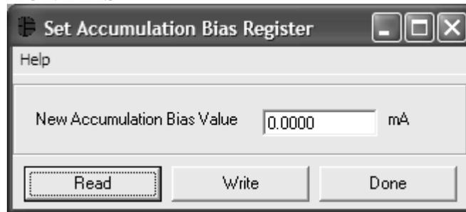
The user can update the Accumulation Bias Register by left clicking on the Update Acc Bias button on the Meters Tab. That will open up the Set Accumulation Bias Register window. When the user left clicks the Write button the value that is entered into the New Accumulation Bias Value text box will be written to the Accumulation Bias Register. This new value will not be added to the current register but will be added to the ACR.
