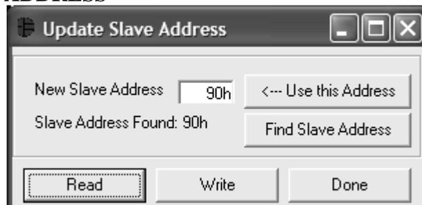
The user can bring up the Update Slave Address window by left clicking the Update Slave Address button of the Meters Tab. This window allows the user to enter a new Slave Address that the software uses for communication, find the first Slave Address that has a responding device on the 2 Wire bus, or
