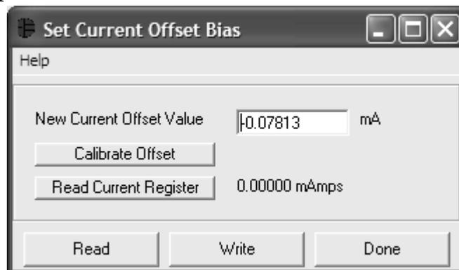
The user can bring up the Set Current Offset Bias Register window by left clicking the Update Offset button of the Meters Tab. The Calibrate Offset button allows the software to auto-detect the appropriate Current Offset Bias Register value based on the Current Reading. The auto-detection should be performed while the pack is disconnected and there is no current flow. The process takes approximately
