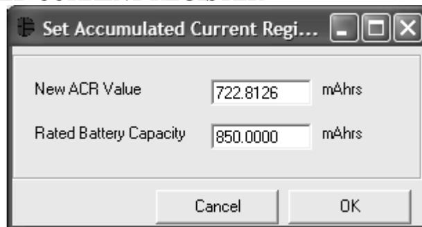
The user can bring up the Set Accumulated Current Register window by left clicking the Set ACR button of the Meters Tab. This window allows the user to enter values for the Accumulated Current Register and Rated Battery Capacity in mAH. Rated Battery Capacity is used to determine full-scale range on the Accumulated Charge Meter. This value is stored in software only and does not affect the Fuel Gauging data.
