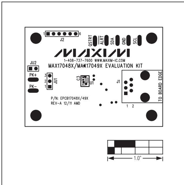
Figure 4. MAX17048X/MAX17049X EV Kits PCB Layout—Component Side
