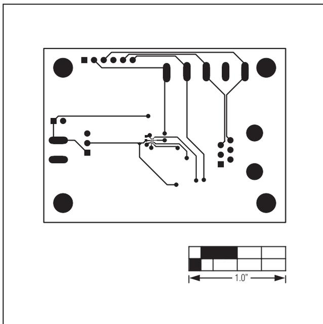
Figure 5. MAX17048X/MAX17049X EV Kits Component Placement Guide—Component Side
