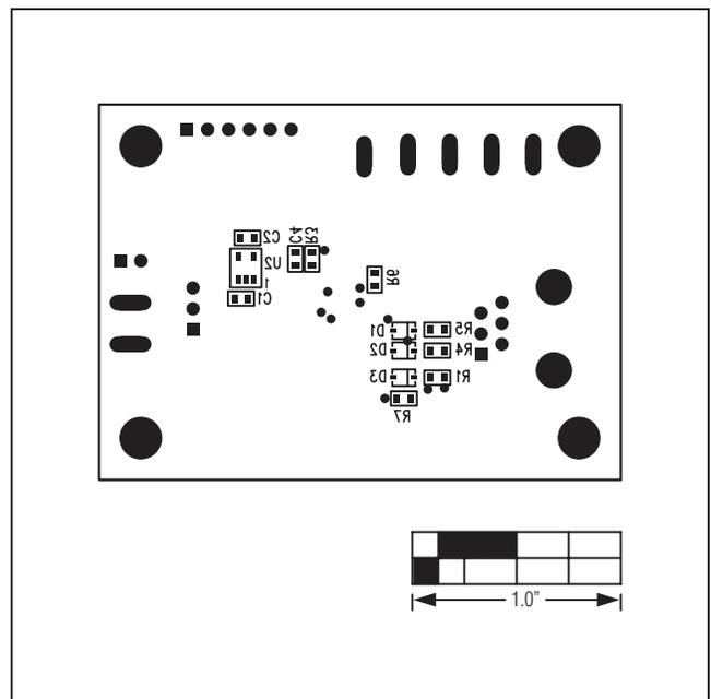
Figure 7. MAX17048X/MAX17049X EV Kits Component Placement Guide—Solder Side
