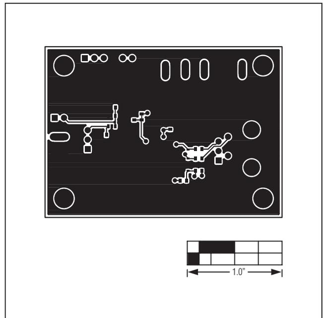
Figure 6. MAX17048X/MAX17049X EV Kits PCB Layout—Solder Side
